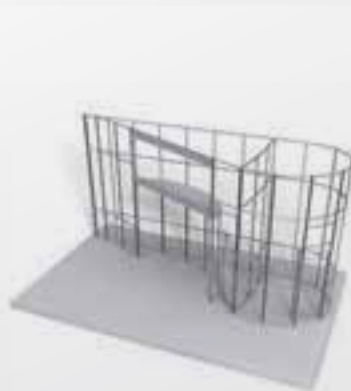
2) Complete the framework to a maximum 4m high
